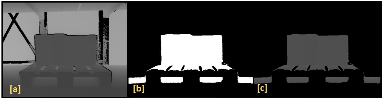
Figure 4: Isolation method applied to range data [depth map]. Source image [a], data within desired depth range [mask][b], isolated depth data using mask [c].
