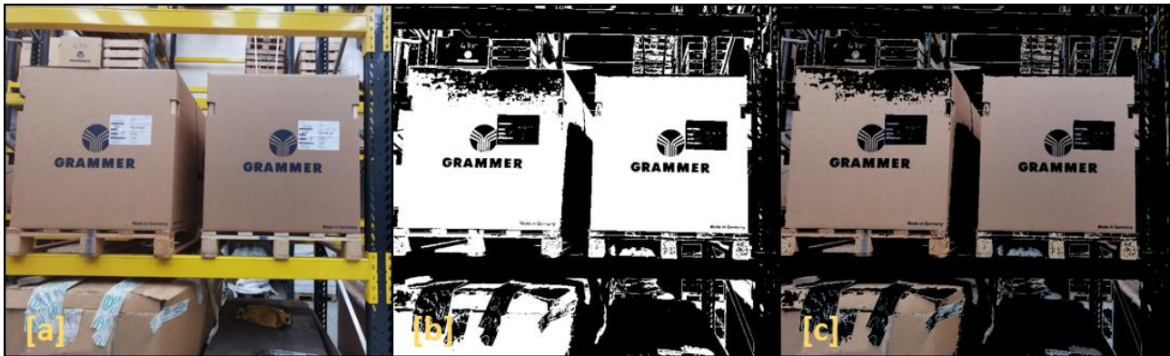
Figure 2: Source image [a], isolated data in desired colour range [mask] [b], mask applied to source data [c].
