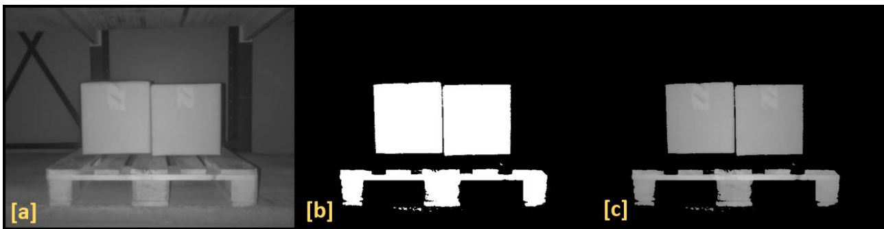
Figure 3: Colour-based isolation method applied to TOF intensity data. Source data [a], threshold data [mask][b], mask applied to source [isolated] data [c].
