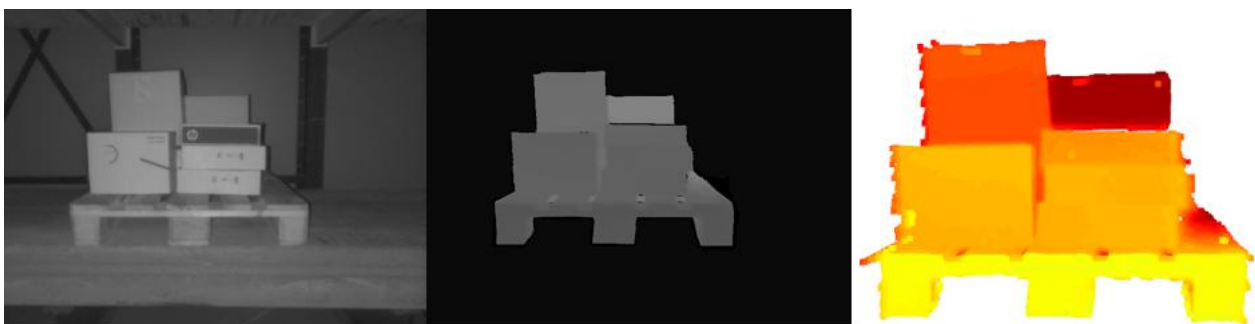
Figure 7: Intensity image of load (left), curated depth map (centre), point cloud of curated load (right).
