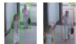
Figure 2: (left) distances are correctly detected (right) the pair are falsely found to be within 2m.
