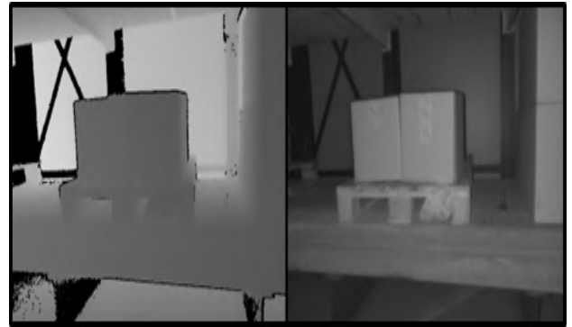
Figure 1: Depth map of scene (left), intensity image of scene (right).
